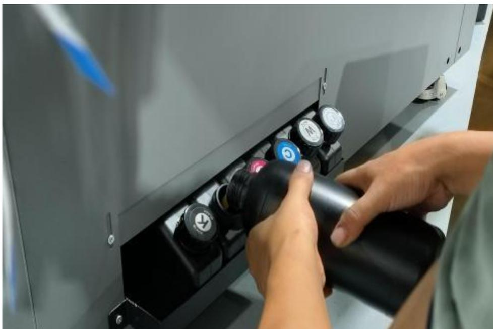
12. Plug in the ink supply line on the headplate in sequence
