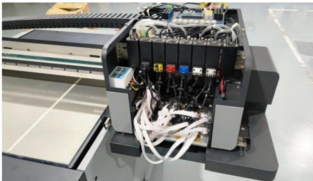
*\*The moving components in UV printers mainly include the print head, motor, and sensor, which we usually refer to as the "ink cart". This word will also appear later .*
