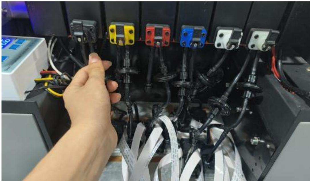
14. After the ink is completed, connect the nozzle and the valve port with the following nozzle sequence
