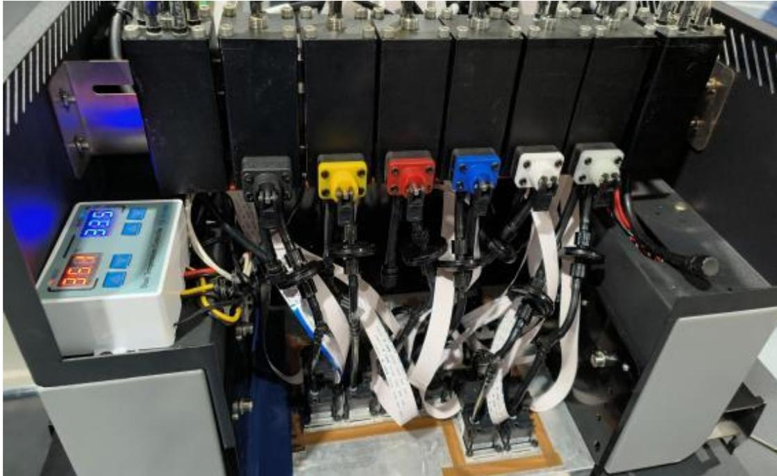
15. After the ink pipe is connected to the secondary ink cartridge, open all the valves and press the ink button to squeeze the ink out of the nozzle. (The valve is open to the right, other positions are closed, and the following figure is the closing direction)
