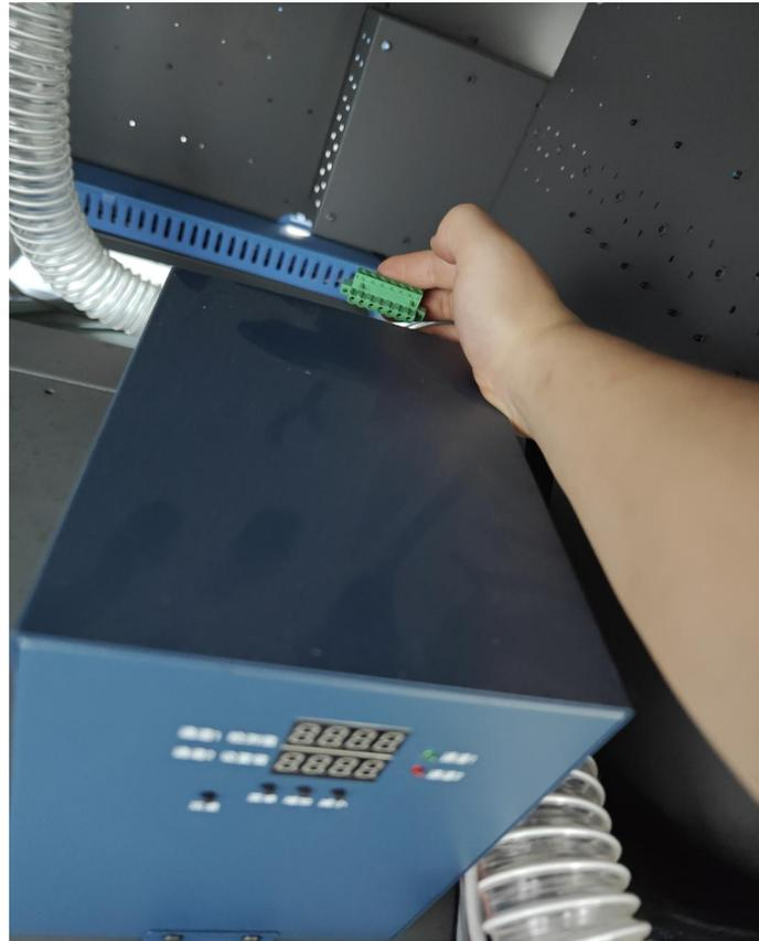
16. Get a bottle Open the secondary cartridge valve Aim the bottle at the ink outlet, then press the ink press switch to squeeze the ink out of the cartridge.
