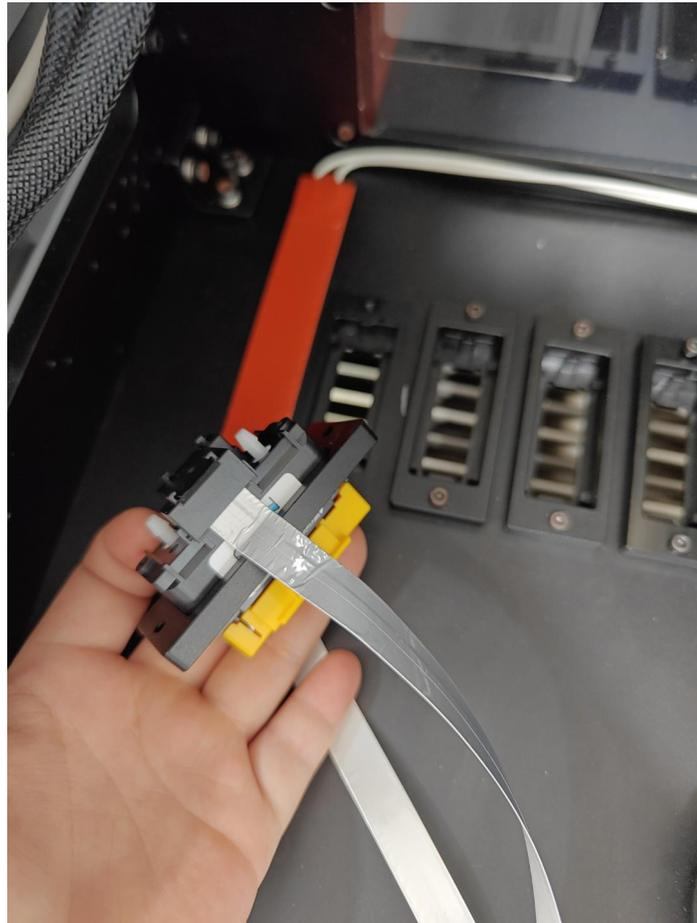
8. Linking the ink tube to the printhead
