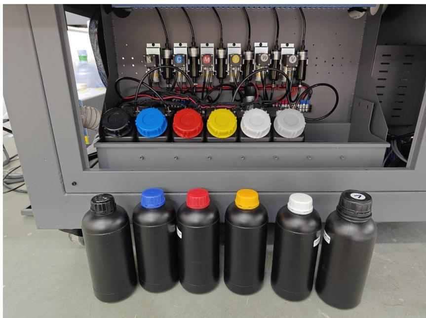
13. Plug in the ink supply lines on the header board in sequential order
