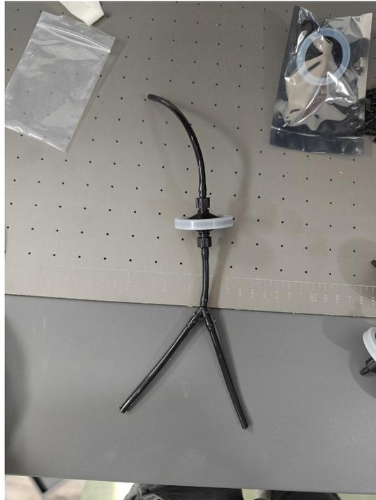
6. Take out the nozzle, open the nozzle cover, install the nozzle line, line, through the nozzle cover, nozzle cover installation back to the nozzle, need to pay attention to, line installed to the nozzle, line insertion method for, blue face inward, metal face outward
