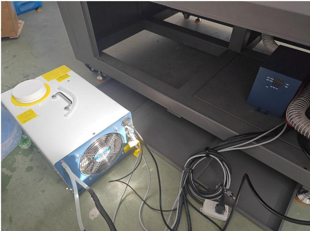
3. Connect the machine to the power supply. Check that the cartridge alarm device is normal. Ink is not refilled at this time.
